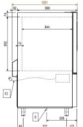
Drain Electrical inlet (power)
